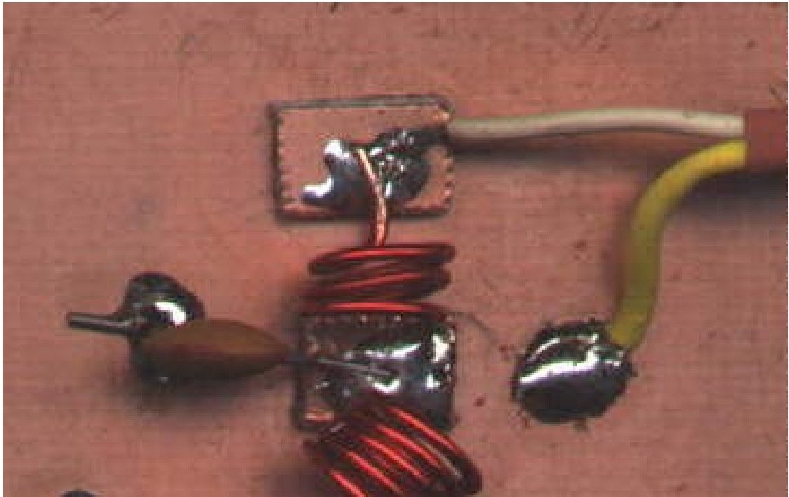
Tie-points are made from 1/4 inch squares of PC board material glued with "crazy-glue" to a solid ground plane of PC board.
